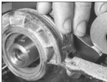
11.8b Lugs of cork gasket halves to fit under the cut-outs in the rubber gaskets
