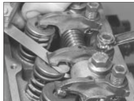
5.6 Adjusting the valve clearances
