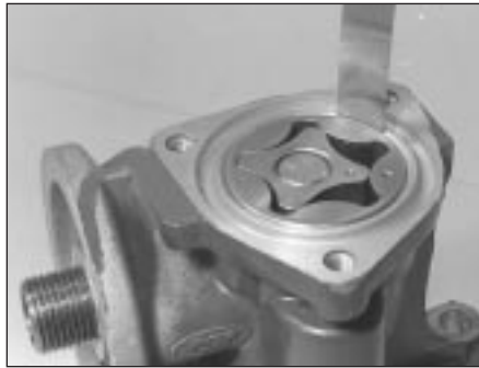
13.4a Checking the outer body-to-rotor clearance
