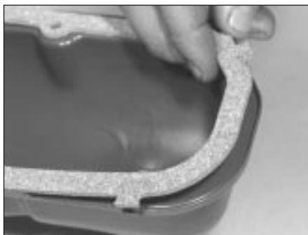
4.6a Engage tags of rocker cover gasket into the cut-outs in the cover
