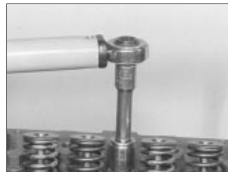
7.27b Tightening the cylinder head bolts (Stage 1)
