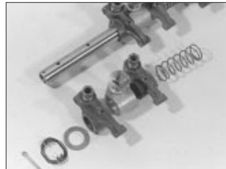
6.4 Rocker shaft partially dismantled for inspection
