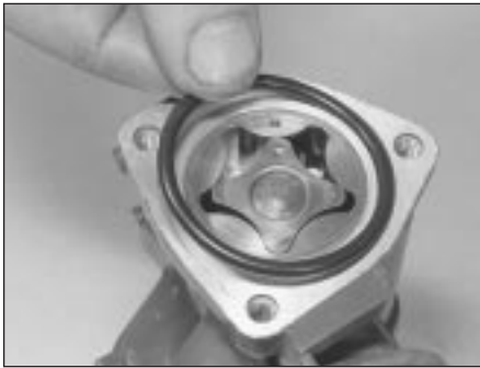
13.1 Extract the O-ring from the groove in the oil pump
